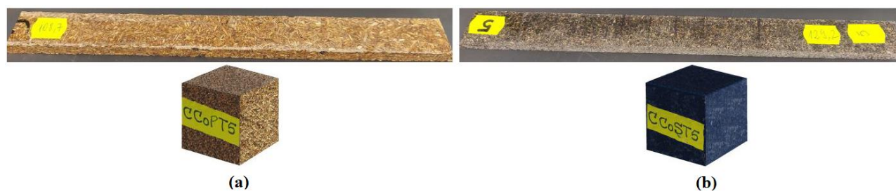
Figure 1. Examples of samples made from the composite materials studied, with shredded wheat straw (a) and sunflower seed hulls (b) as reinforcing material, subjected to various mechanical stresses
